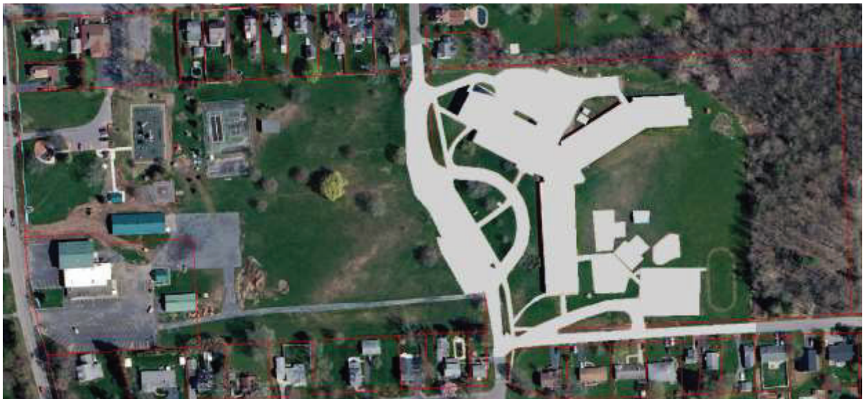
Impermeable Town roads and structures at the Owasco Elementary School in grey.
